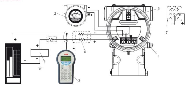
HART hand-held communicator may be connected at any wiring termination point in the loop, providing the minimum resistance is 250 ohm. If this is less than 250 ohm, additional resistance should be added to allow communications. Maximum voltage drop on external remote indicator is 0.7 Vdc
