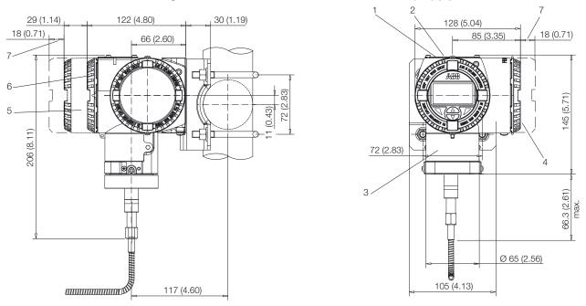
1 Adjustments | 2 Identification plate | 3 Certification plate | 4 Terminal side | 5 Integral display housing | 6 Electronic side | 7 Space for cover removal
